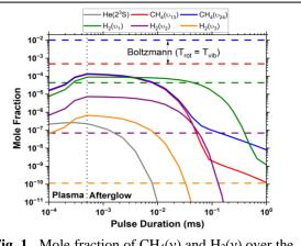
**Fig. 1**. Mole fraction of  $CH_4(v)$  and  $H_2(v)$  over the duration of a quasi-steady state pulse (dashed line represents Boltzmann distribution at  $T_{vib} = T_g$ )
